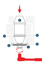
1. Retain the spacer ring of the joint if present. If a spacer ring (5) is supplied with the Hjo Bultens expander bolt, place this on the shoulders opposite side between the bearing inner track and the fixing lug. Make sure that the beveled side of the ring is facing the bearing. Also fit shims (11).
