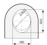
4. Check that the wear – difference between the bolts diameter and bearings diameter in the worn hole – do not exceed 2 mm\*. In other cases you must use oversized bushings.
