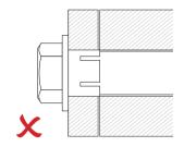
If the coaster washer contacts the fixing lug, the conical bushing is not correctly matched. You must then use an oversized conical bushing. Contact your retailer or Hjo Bulten Phone: +46 142 42 200.
